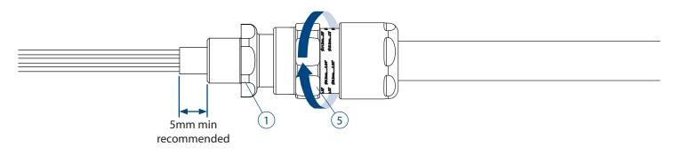
**NOTE:** Support the cable to prevent it twisting. To aid wiring inside the enclosure, it may be beneficial to strip the inner sheath as shown above.
